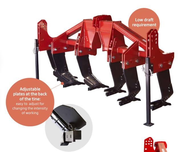
The six tines of the Agrolux EVO Grubber 3.0 are mounted in V-shape for easy releasing residues.
